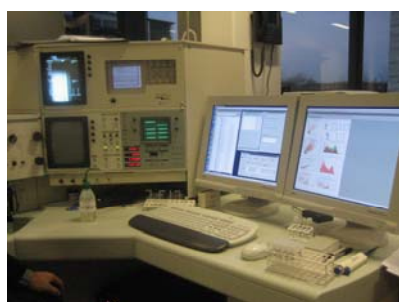
Figure 3. Left: The image shows the Becton Dickinson FACS Vantage used in the routine analytical testing for IC2 autoantigen expression in vitro . This device is also applicable for specific preparative sorting of beta-cells from dispersed splitase/accutase dissociated islet cells. Right: Flow cytometric analysis with glucose sensitive RIN-5AH beta-cells stained indirectly at low glucose concentration (5 mM, red curve) and at high glucose concentration (12 mM, black curve) with IC2 followed by anti-rat IgM-Alexa 488. The blue top represents the isotype control rat IgM. Note that the 2 decades stronger binding of IC2 in comparison to control, with 1 decade increase in IC2 expression after glucose stimulation, is an indication of the functional state-dependent expression of the cell surface IC2 autoantigen.
